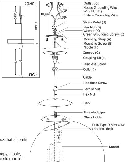
1. Carefully remove the fixture from the carton and check that all parts are included.
